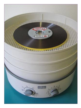
6 dehydrators were in simultaneous use. 3 tapes per unit were dried at the same time, making a total of 18 tapes per day. We treated the tapes for 2 hours on one side, 2 hours on the other side, at 55 degrees Celsius. This process rendered playable tapes for digitization.
