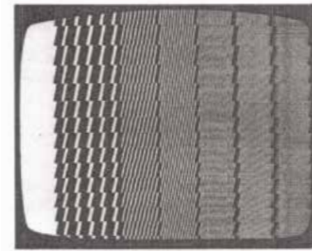
Figure 16—Jogs in Bar Pattern, Insufficient Head Penetration
