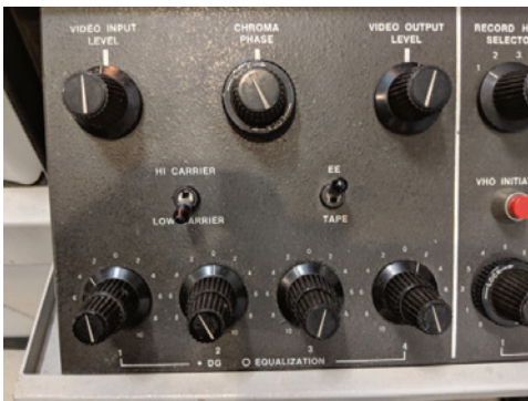
Figure 11. Knobs that control the settings on an Ampex quad VTR. Differential gain (DG) and equalisation settings are critical controls to minimize or prevent “banding” in the picture, as shown in figure 12.
