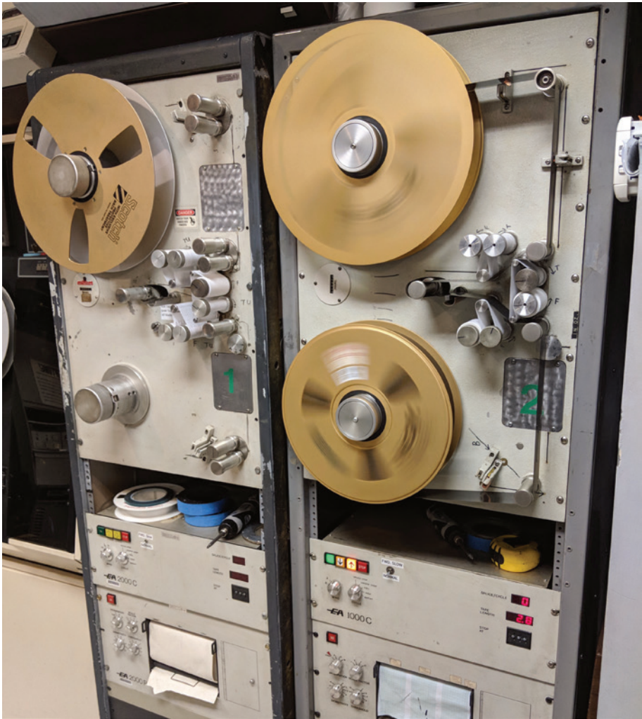
Figure 6. Tape cleaning devices for 2-inch magnetic tape. In the rack below the operational part of the cleaning device are evaluators that prepare and print out reports on the cleaning process, offering an assessment of the tape's condition.
