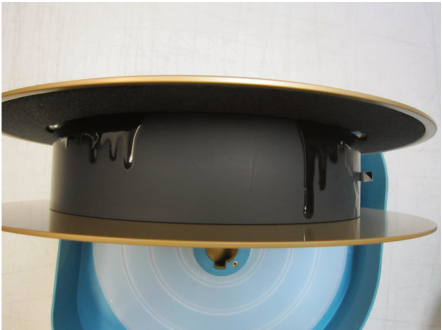
Figure 4. Severe case of foam flange glue failure.
