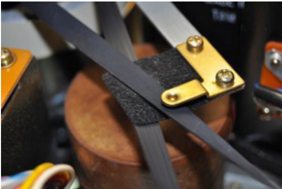
C.3 Figure 6. Cross-over belt and anti-static mechanism inside a 1/2-inch open reel VTR.
