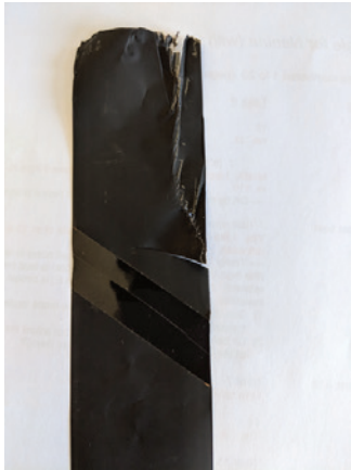
Figure 15. Quad tape sliced by heads after encountering an incorrectly made splice.
