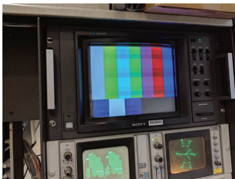
Figure 12. Video monitor showing bands that result from improper equalisation between the heads.
