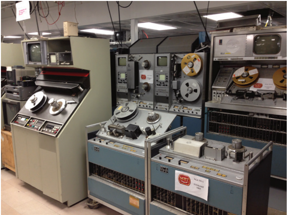
Figure 8. Representative RCA quadruplex recorders at the Museum of Broadcast Technology in Woonsocket, Rhode Island.
