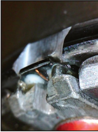
Figure 10. One of four heads on the headwheel.
