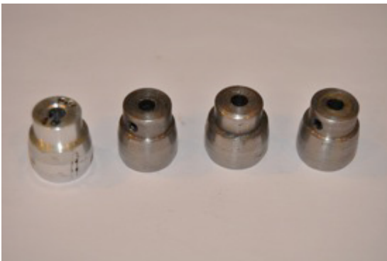
C.3 Figure 5. Capstan and drive for 1/2-inch VTR, with custom replacement capstans. Top: internal view of 1/2-inch VTR, showing capstan pulley and drive belt; bottom: set of custom-machined capstan pulleys in slightly different diameters.
